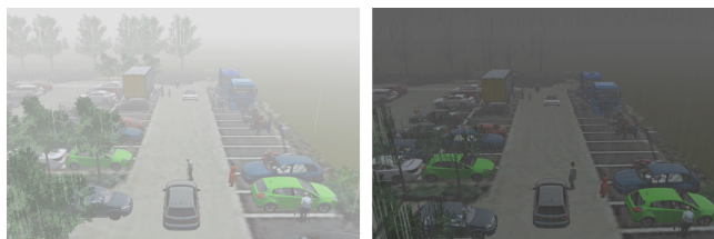
Fig. 10: Critical test cases generated for the AVP system in the pedestrian-avoiding scenario, including a rainy and foggy case ( left ) and a rainy and dark case ( right ).
